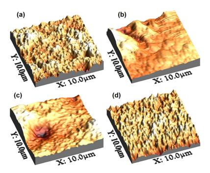
Figure 3. AFM images of (a) MoO<sub>3</sub>/PEDOT:PSS, (b) MoO<sub>3</sub>/PEDOT:PSS-A organotin (IV), (c) MoO<sub>3</sub>/PEDOT:PSS-B organotin (IV) and (d) MoO<sub>3</sub>/PEDOT:PSS-C organotin (IV) films.
