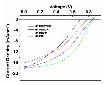
**Figure 11.** Current density–voltage curves under 100 mW/cm<sup>2</sup> AM 1.5G illumination for hybrid photovoltaic structures using pristine PEDOT:PSS film post-treated IPA PEDOT:PSS films using VAPOR, DROP, and DIP techniques.
