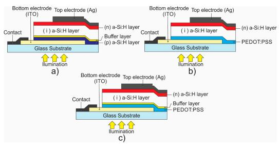
**Figure 1.** Schematics of (a) photovoltaic structure based on amorphous silicon (a-Si:H reference sample), (b) superstrate-type hybrid structure (H1) with PEDOT:PSS/a-SiH heterojunction in frontal interface, and (c) superstrate-type hybrid structure (H2) with PEDOT:PSS/buffer/a-SiH heterojunction in frontal interface.
