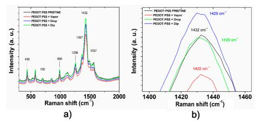
**Figure 9.** (a) Raman spectra of pristine PEDOT:PSS film post-treated IPA PEDOT:PSS films using VAPOR, DROP, and DIP techniques. (b) Close view of Raman band associated to C=C symmetrical stretching intramolecular vibration of PEDOT between 1400 and 1460 cm<sup>-1</sup> (benzoid/quinoid forms).
