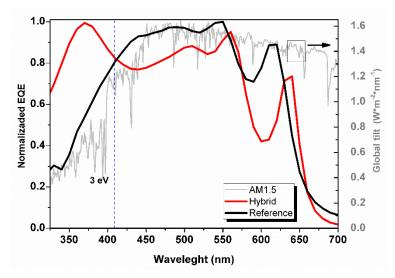
**Figure 12.** (a) External quantum efficiency (EQE) spectra of a photovoltaic structures based on amorphous silicon (a-Si:H) (REFERENCE) and a hybrid photovoltaic structure with a buffer layer and a PEDOT:PSS film treated with DIP in IPA (H6-DIP). (b) Comparison of EQE spectra in the range from 300 nm to 450 nm obtained using both LED and GLOBAL source.
