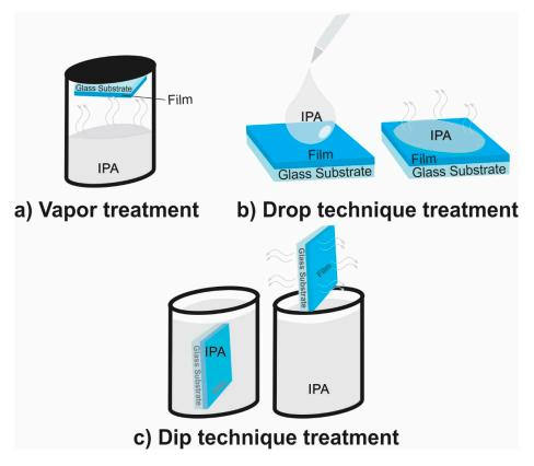
**Figure 2.** Schematic illustration of different solvents treatments used in this work: (a) vapor, (b) drop, and (c) dip techniques.
