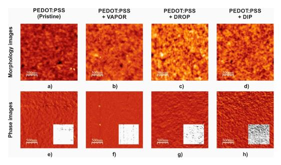
**Figure 7.** Atomic force microscopy (AFM) (morphology and phase) images of (**a**) and (**e**) pristine PEDOT:PSS film post-treated IPA PEDOT:PSS films using (**b**) and (**f**) VAPOR, (**c**) and (**g**) DROP, and (**d**) and (**h**) DIP techniques; high-contrast phase images (inset images)
