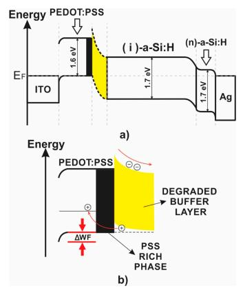
**Figure 4.** (a) Energy level band diagram in thermal equilibrium for a hybrid structure and (b) schematic representation of the electron-blocking mechanism with the buffer layer (SIC:H/Si:H) by interfacial wide energy gap PSS [26].
