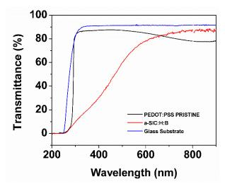
**Figure 5.** Optical transmittance spectra of an amorphous silicon carbine film doped with boron (a-SiC:H:B), PEDOT:PSS pristine film, and glass substrate.
