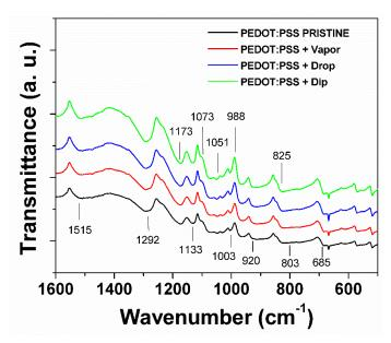
**Figure 8.** Fourier-transform infrared spectroscopy (FTIR) spectra of pristine PEDOT:PSS film post-treated IPA PEDOT:PSS films using VAPOR, DROP, and DIP techniques.
