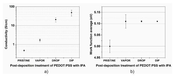
**Figure 6.** (a) Electrical conductivity and (b) work function of pristine PEDOT:PSS film and post-treated IPA PEDOT:PSS films using VAPOR, DROP, and DIP techniques.
