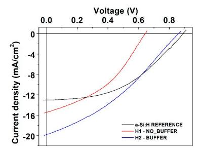
**Figure 3.** Performance parameters of hybrid photovoltaic structures fabricated with pristine and post-treated PEDOT:PSS films.
