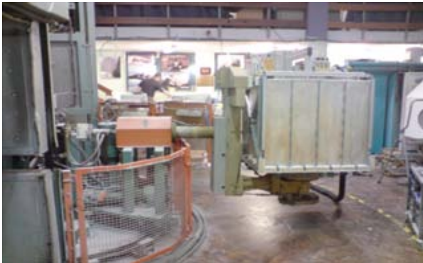
FIGURE 2 – PROTOTYPE MICROWAVE OVEN ON DROP ARM OF ROTOMOULDING MACHINE
