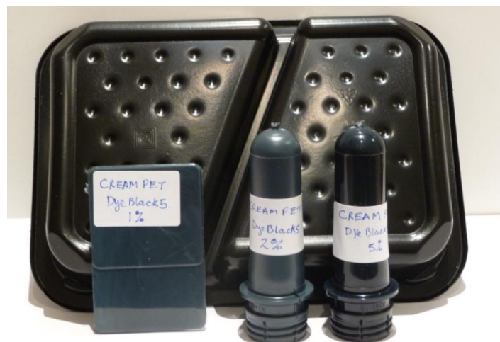
Figure 7. 100% Cream/ivory CPET regrind mixed with ColorMatrix Dye Black-5 at (l-r) 1%, 2% and 5% addition rate. The carbon black tray in the background is used for comparison.
