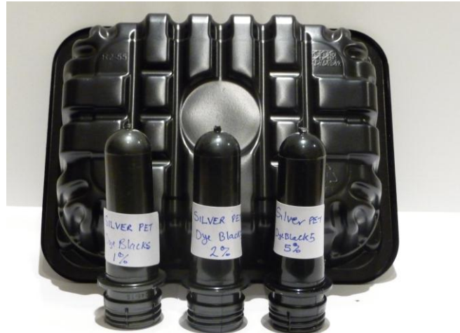
Figure 8. 100% Silver APET regrind mixed with 1.0, 2.0 and 5.0% Dye Black-5. A carbon black tray in the background is for comparison.
