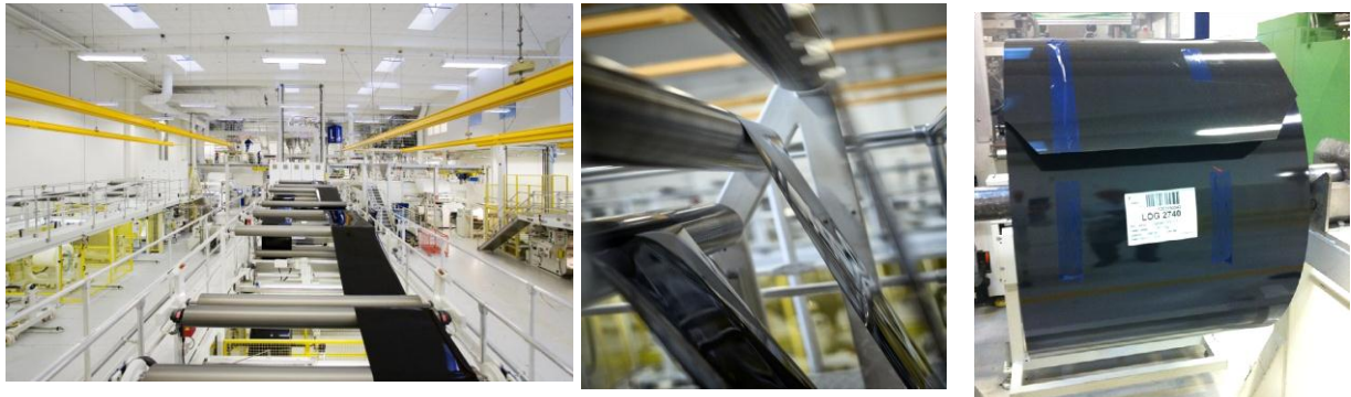
Figure 17. Images from CPET multi-layer sheet extrusion trials at Færch Plast.
