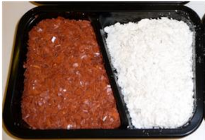
Figure 1. Example of the terracotta and ivory CPET regrind supplied by Færch Plast.
