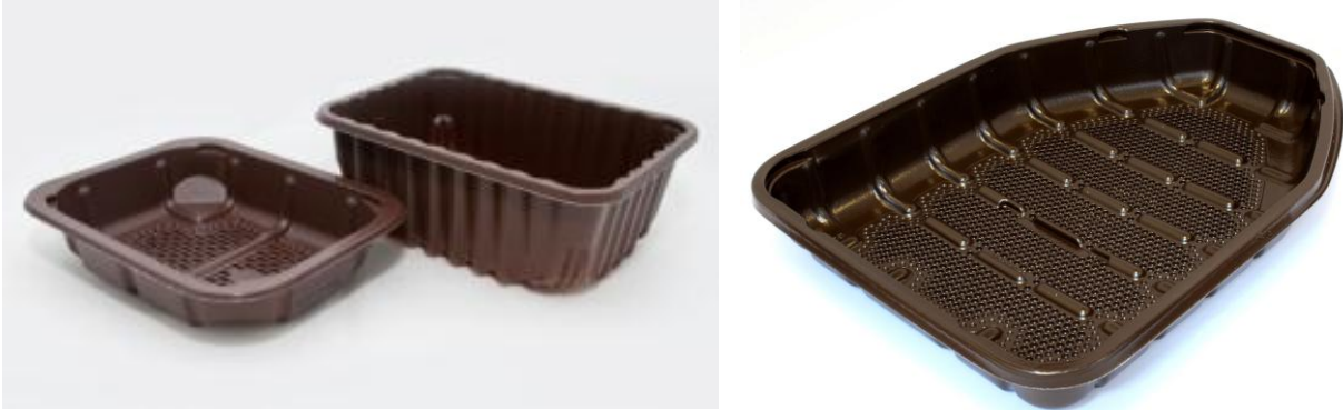
Figure 15. PP trays showing the influence of 2% masterbatch addition rate of the IRR 95530 detectable black colourant. Standard brown products are shown on the left and the effect of additional black is shown on the right
