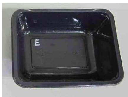
e) Detectable black 70 micron layer (front) and standard CPET(back).Sample E was water/heat treated
