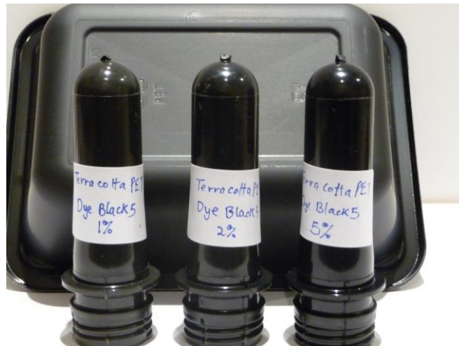
Figure 9: 100% Terracotta CPET regrind mixed with 1.0, 2.0 and 5.0% Dye Black-5. A carbon black tray in the background is for comparison.
