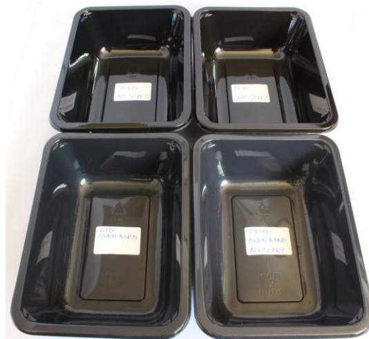
Figure 20. Examples of standard (carbon black) and trial CPET trays before and after oven ageing, showing a level of greying due to crystallisation.
