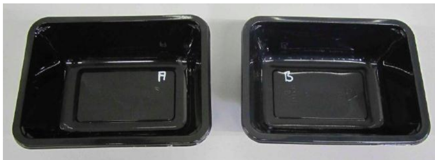
a) Detectable black 70 micron layer (front) and standard CPET (back) – standard tool sample
