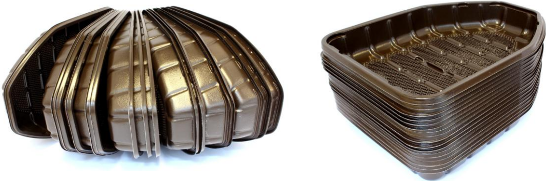
Figure 16. Example of stacked trays showing the lack of masking achieved on the brown colour.
