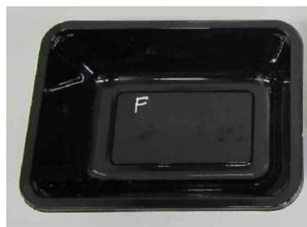
f) Standard APET (front) CPET (back) with carbon black. Sample F was water/heat treated.
