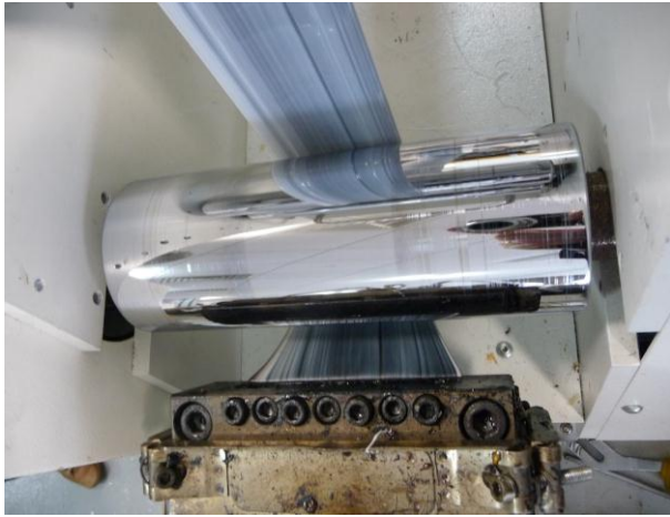
a) example of the white PP middle layer in the process of being coated with a detectable black layer.
