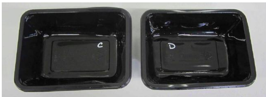
c) Detectable black 70 micron layer (front) and standard CPET (back). Sample C was heat treated
