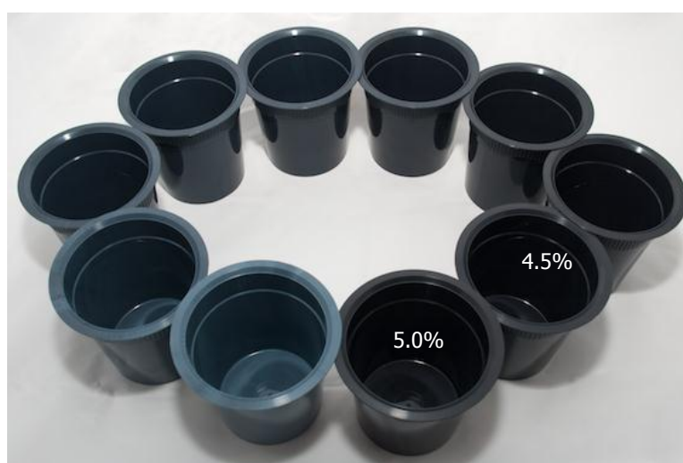
Figure 14. The samples show the variation in masking strength capability of Colour Tone IRR 95589 at addition rates of 0.5% to 5.0%
